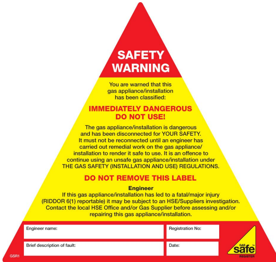
Figure 6 - Typical 'Immediately Dangerous' Warning Label (approximately - 150mm (H) x 160mm (W))
